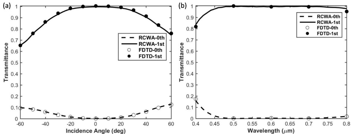
Figure 5. (a) Angular response of achromatic PG at 532nm, (b) Spectral response of achromatic PG at normal incidence.
