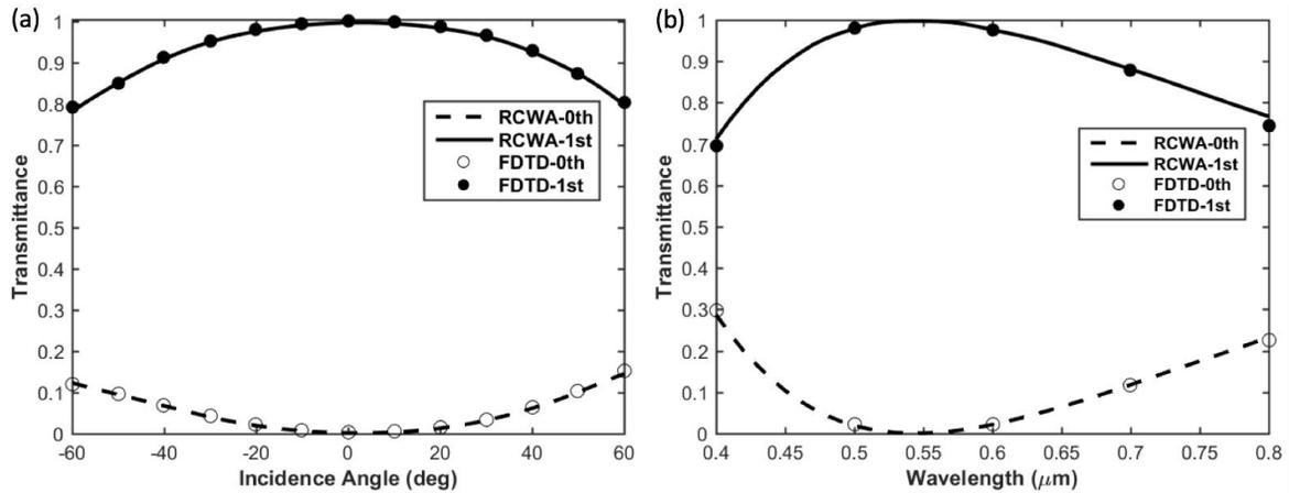
Figure 4. (a) Angular response of non-twist PG at 532nm, (b) Spectral response of non-twist PG at normal incidence.
