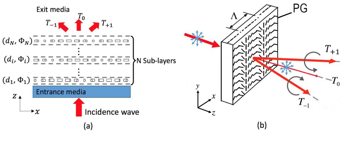
Figure 3. (a) Illustration of  $N$  sub-layers for a multi-two-twist, (b) Polarization dependence of diffraction orders.
