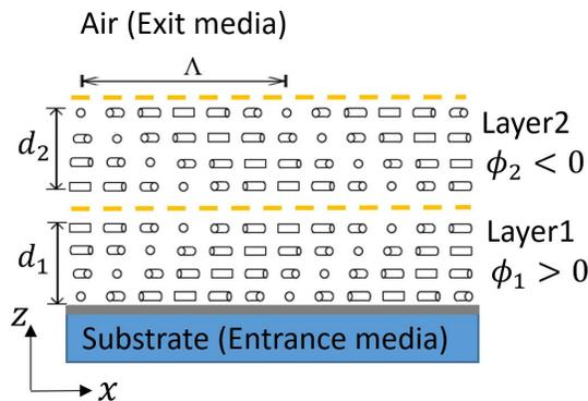
Figure 2. The structure of a typical two-twist achromatic PG. QUESTION: does this Fig. 2 correctly represent the algorithm? i.e., the user defines layer 1 and 2 from substrate up, and then the simulation has light incident from layer 2 into 1 into the substrate? If so, this would be best.]]
