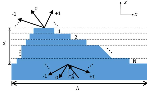
Figure 1. Geometry for a generic (isotropic) surface-relief grating. Transmitted and reflected diffraction orders are also shown.
