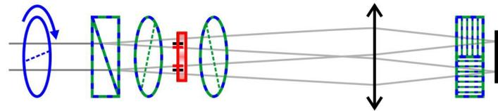
2D vAPP with leakage filtering and 2x single-beam polarimetry, v2
