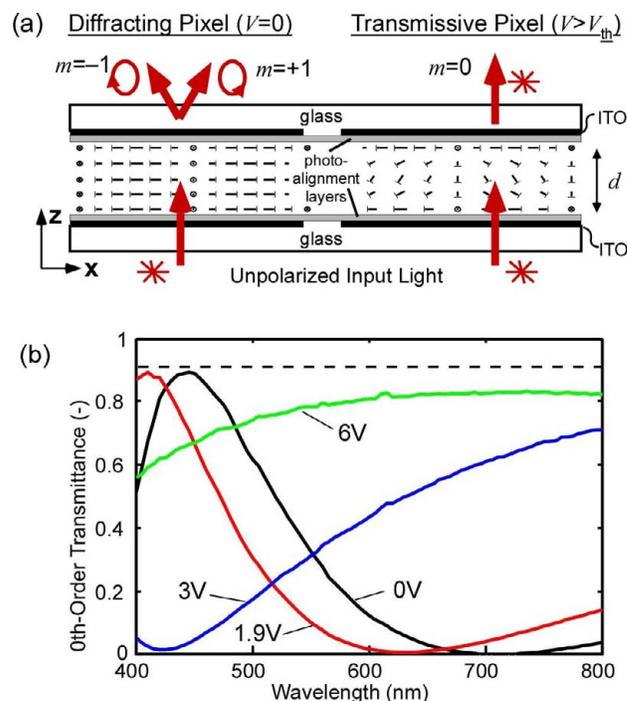
**Figure 1: LCPG properties - (a) Side-view of the pixel structure in its diffracting and transmissive states; and (b) raw transmittance of the 0<sup>th</sup> order with input unpolarized light. Note the blue-shift of the spectra as voltage is applied.**
