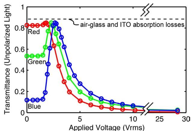
Figure 5: Dark-field Schlieren projected transmittance for red, green, and blue LEDs.
