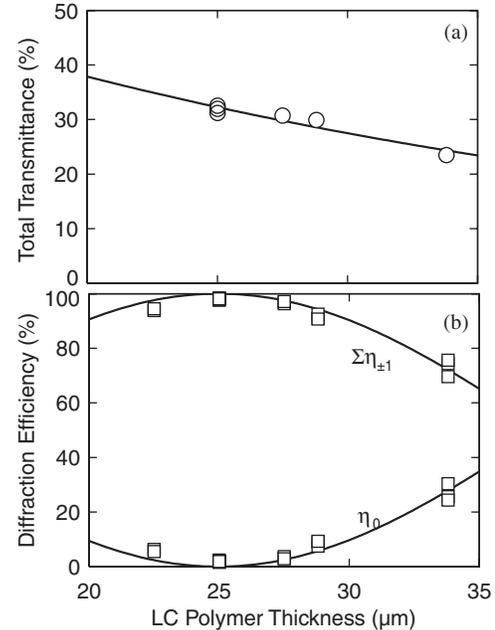
FIG. 5.—Measured MIR narrowband PG throughput at  $10.6 \mu\text{m}$  laser wavelength: (a) total transmittance into any forward direction and (b) diffraction efficiency of first and zero orders. Note that discrete points are measured data, while curves are theoretical fits employing eqs. (1) and (5).
