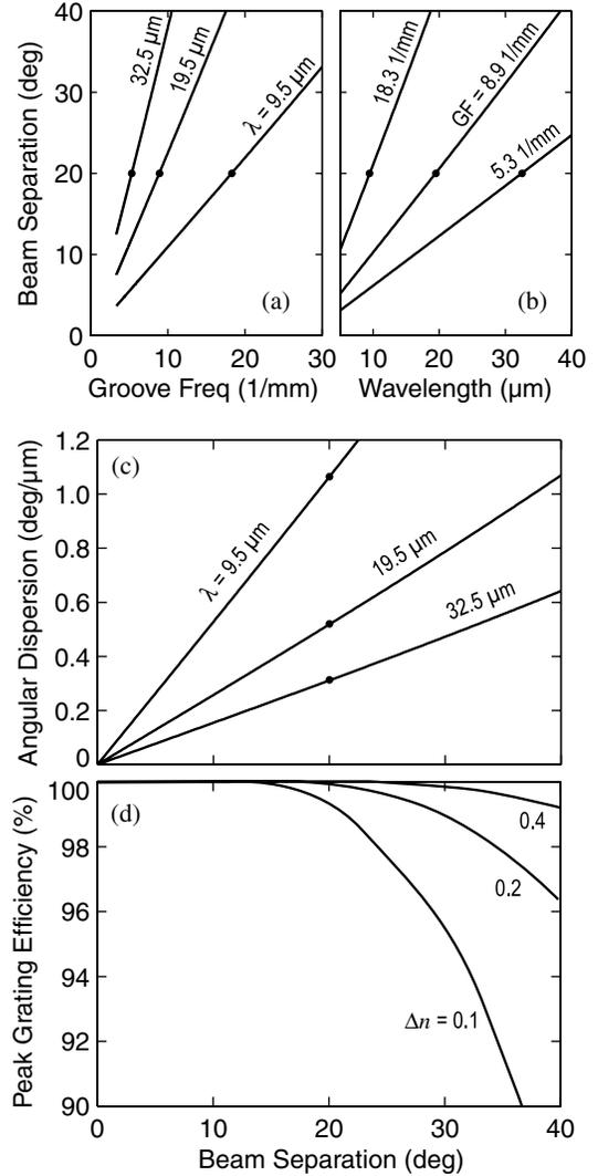
FIG. 6.—PG diffractive beam splitting characteristics: (a)–(b) beam separation between the +1 and –1 diffraction orders, for several  $\lambda$  and GFs, (c) angular dispersion, as governed by the grating equation, and (d) peak first-order efficiency for several values of birefringence  $\Delta n$ , as calculated using finite difference time-domain numerical simulation (Oh & Escuti 2006). Note that the discrete points correspond to the design points in Table 2 and surrounding discussion.
