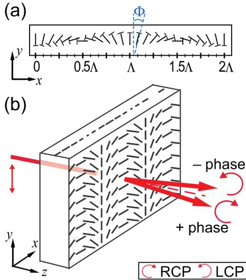
Fig. 1. PG structure, with an in-plane optical axis (small lines) profile whose orientation angle varies linearly. (a) Plan view. (b) Perspective view, showing linearly  $p$ -polarized input transferred into two parts: RCP with positive phase change and LCP with negative phase change.
