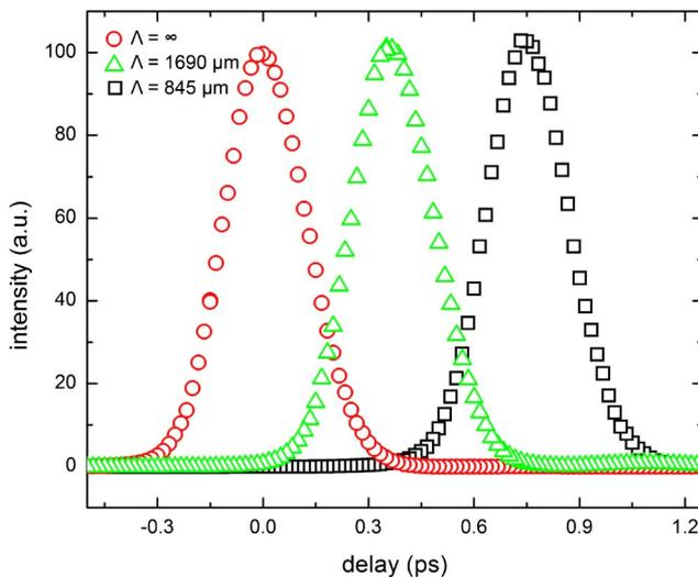
Fig. 4. Delay of LCP pulses using PGs with different grating periods. The PG with  $\Lambda = \infty$  is a half-wave plate that introduces same phase for all frequencies. Hence it does not result in a delay.
