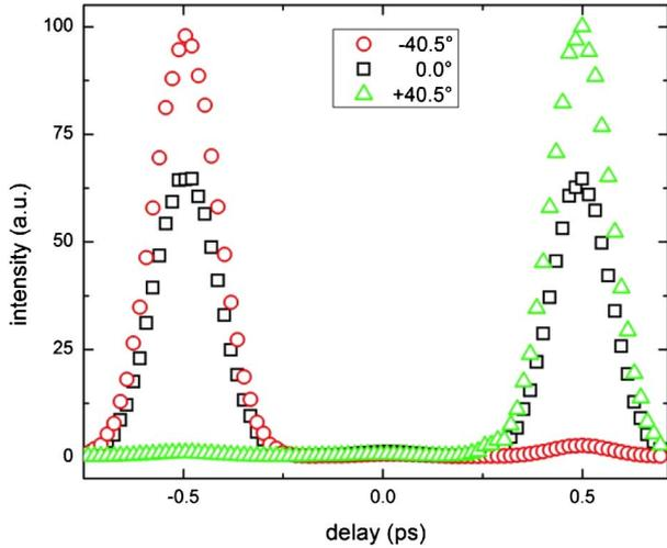
Fig. 3. Cross-correlation of shaped pulses measured by SFG with a reference pulse in a BBO crystal. Type I phase matching only allows  $p$ -polarization to mix with the reference pulse. By setting the QWP to  $\pm 40.5^\circ$  the two orthogonally polarized pulses at delays  $-0.5$  ps (circles) and  $0.5$  ps (triangles) are measured. At  $0^\circ$  QWP setting both pulses partially mix with  $p$ -polarized reference pulse (squares).
