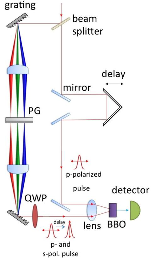
Fig. 2. Experimental setup of PG-based pulse shaper. Femtosecond  $p$ -polarized pulses are chromatically dispersed and focused onto a PG positioned at the Fourier plane. The output is collected and combined with a time-delayed reference pulse for analysis by a BBO crystal and photodetector.
