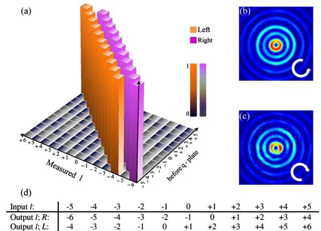
Fig. 5. (a) Correlation signals for the azimuthal decomposition for both the left- (orange) and right-circular (pink) polarization components. (b)  $\ell = +1$  and (c)  $\ell = -1$  Bessel beams after the  $q$ -plate associated with left- and right-circular polarization components, respectively. (d) A table summarizing the transformation of the input  $\ell$  values after the  $q$ -plate.
