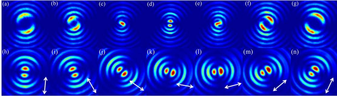
Fig. 4. (a)–(g) Experimentally recorded near-field intensity profiles of vector Bessel fields recorded after the  $q$ -plate with a polarizer in front of the CCD for initial scalar Bessel beams of  $\ell = -5, -3, -1, 0, +1, +3$ , and  $+5$ , respectively. (h)–(n) Intensity profiles for an  $\ell = 0$  vector Bessel beam recorded with a rotating polarizer. The full data (video) can be viewed in [Media 1](#). White arrows mark the corresponding polarizer setting.
