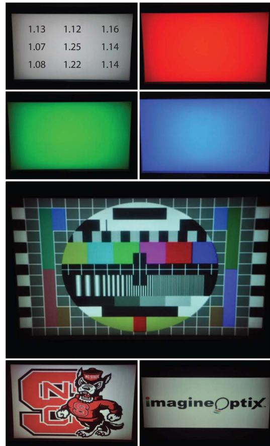
Fig. 7. (Color online) Photographs of images projected by the prototype picoprojector using the PG-PCS.
