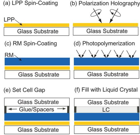
Figure 3. Basic fabrication steps for the BPG
