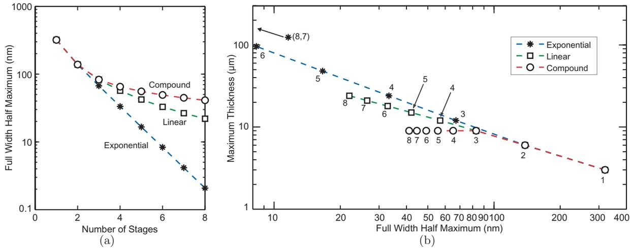
Figure 6. Simulated diffraction characteristics of LCPGs versus number of stages  $M$ : (a) Full-width at half-maximum and (b) Maximum required LCPG thickness and FWHM (numbers indicate  $M$  for each point)<sup>30</sup>
